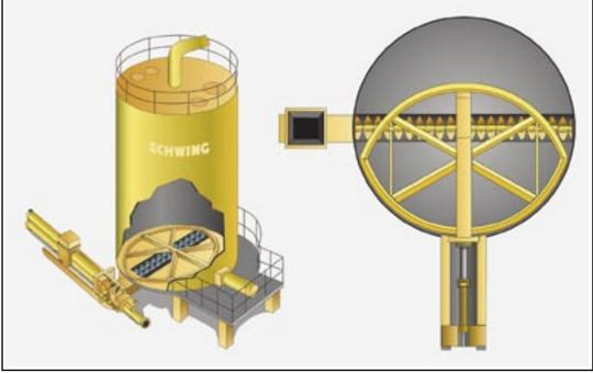
The Push floor rectangular bunker design consists of a series of hydraulically driven push frames (or ladders) that reciprocate along the bunker floor. Each push frame is located on the bearing beams running the length of the installation; they terminate at a cross beam to which the hydraulic cylinders are attached. The
