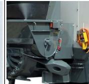
Rock valve in HP design with reinforced agitator.
