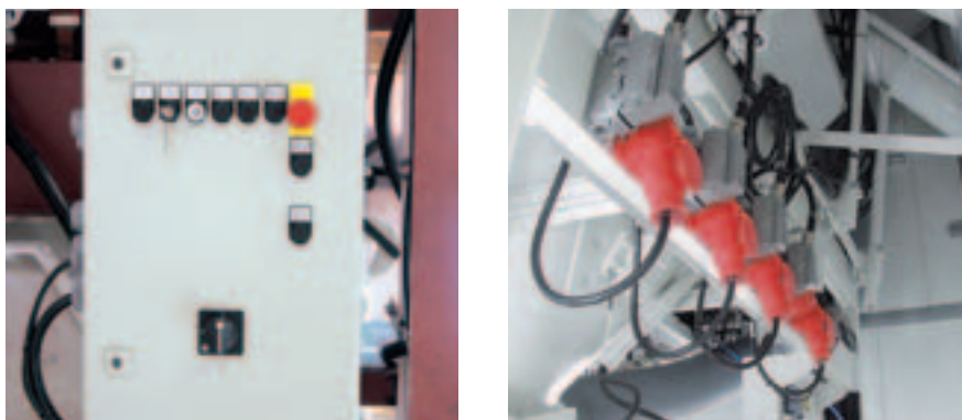
Plug-in connectors for the electrical connection of the peripheral devices make assembly and disassembly operations easier.
