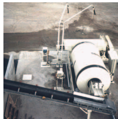
Design with conveyor belt for extracting solids.
